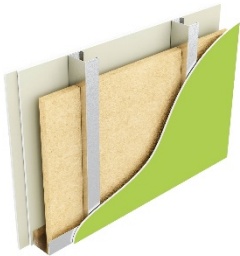
Steel Frame walls (SFS)
