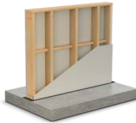
Timber Frame Walls
