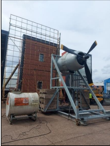
Photograph No. 2 – Hose Fan Test
