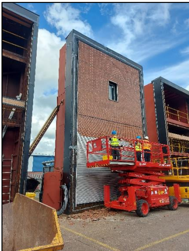
Photograph No. 17 - Sample with bricks partially removed
