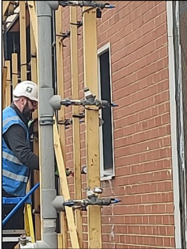
Photograph No. 2 – Hose Fan Test
